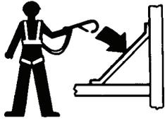
Occupants must wear a safety belt or harness in accordance with governmental regulations. Attach lanyard to anchor provided in platform.
